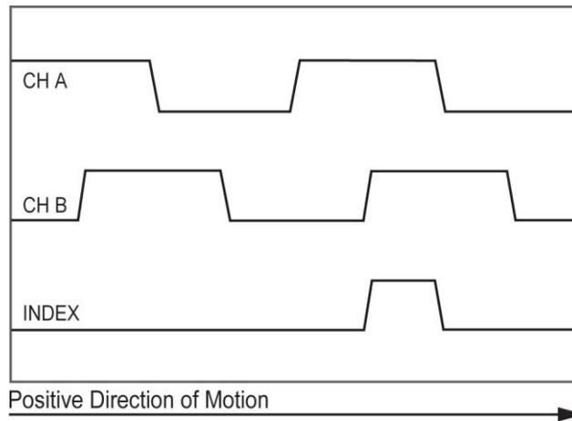
**Figure 7-3: Timing diagram for the encoder signals**
