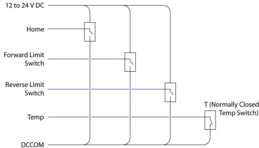
**Figure 7-4: Equivalent Limit, Home, and Temp circuit schematic**
